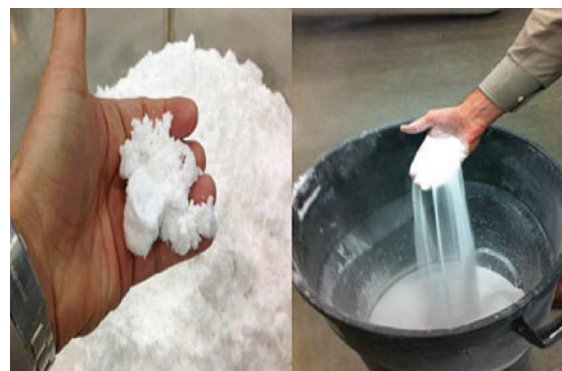
Figure 7: From feedstock to free-flowing finished product through LP flash evaporation
